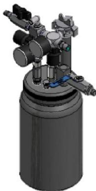
The DBH-01 material pressure tanks made of stainless steel are deliverable in 2l content. The pressure tanks are equipped with a lid with dual cover gasket onto which all fittings such as pressure reducer, safety valve and stopcocks, etc. are mounted. The application valve is fed with the application medium (tank pressure = 0 – 2.5 bar adjustable), atomizing air (0 – 6 bar adjustable) and control air (6 bar).
